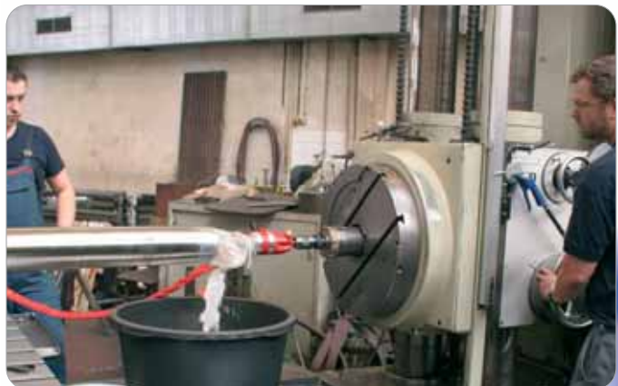
Erosion of the broken drill using the machine's normal cooling fluid
