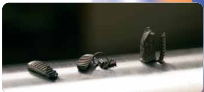
Removed residues of the eroded tool / thread tap
