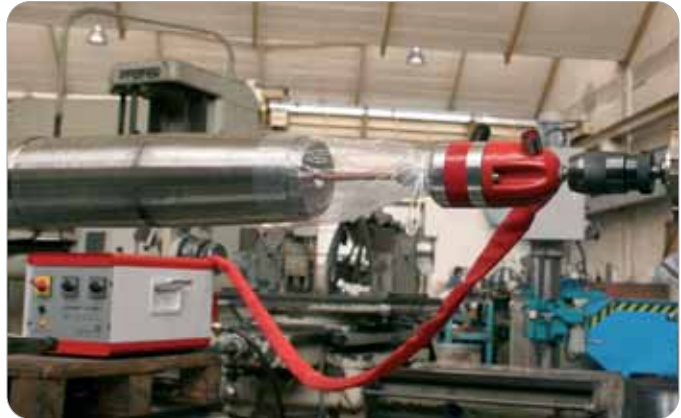
Instead of the tap, the oscillating head of the erosion unit is clamped in the machine
