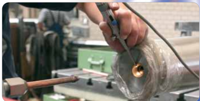
The deep-hole inspection light is used to check for remaining tool residues
