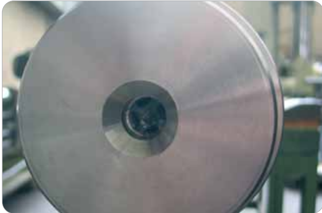
Shaft containing a snapped-off 3/8 inch thread tap
